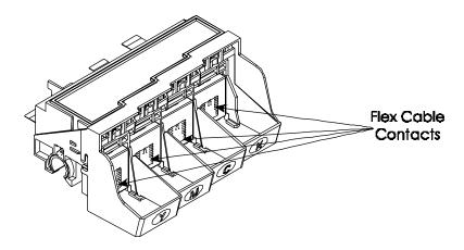
Figure 3-3. Flex Cable Contacts.
